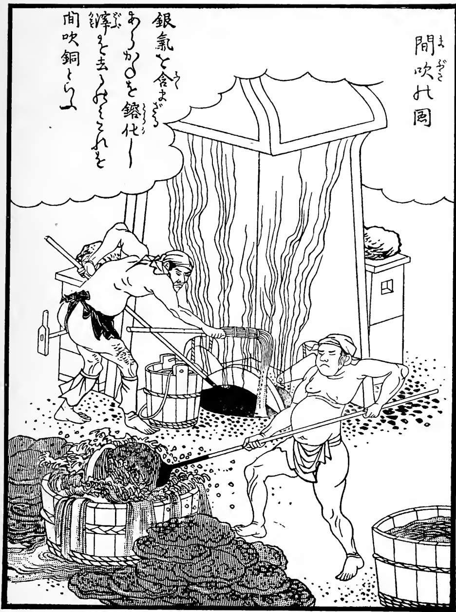
REMOVING THE COPPER FROM THE SMELTING FURNACE.
